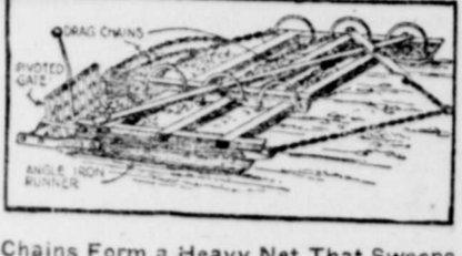
Chains Form a Heavy Net That Sweeps the Roads for Stones.
