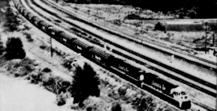
The modern 100-ton jumbo covered hopper can be loaded with wheat in about twelve minutes and unloaded in less than three.
