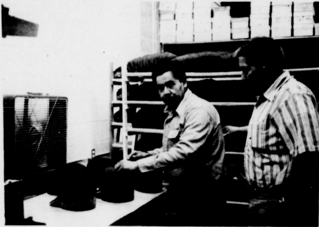
BLOCKING CAPS —Gilbert Torres, left, is pictured above as he blocked new caps coming off the production line at the Crowell cap factory. This is the last process before the caps are boxed for shipment. On the right is Joe Ray Setliff, plant manager.
