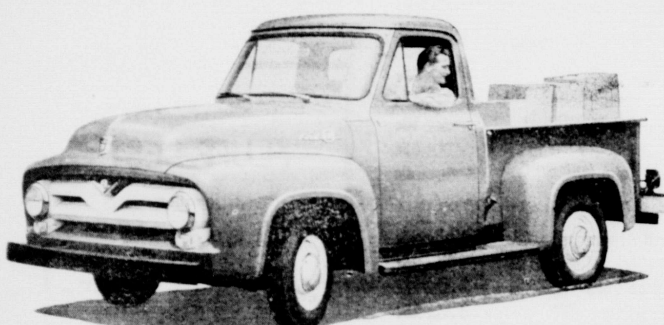
Ford 6 1/2 T Pickup gives choice of Short Stroke 132 h.p. V-8 or Short Stroke 118 h.p. Six. Tubeless tires standard. Fordomatic Drive and Power Brakes available at low extra cost. GVW 3,000 lbs.
