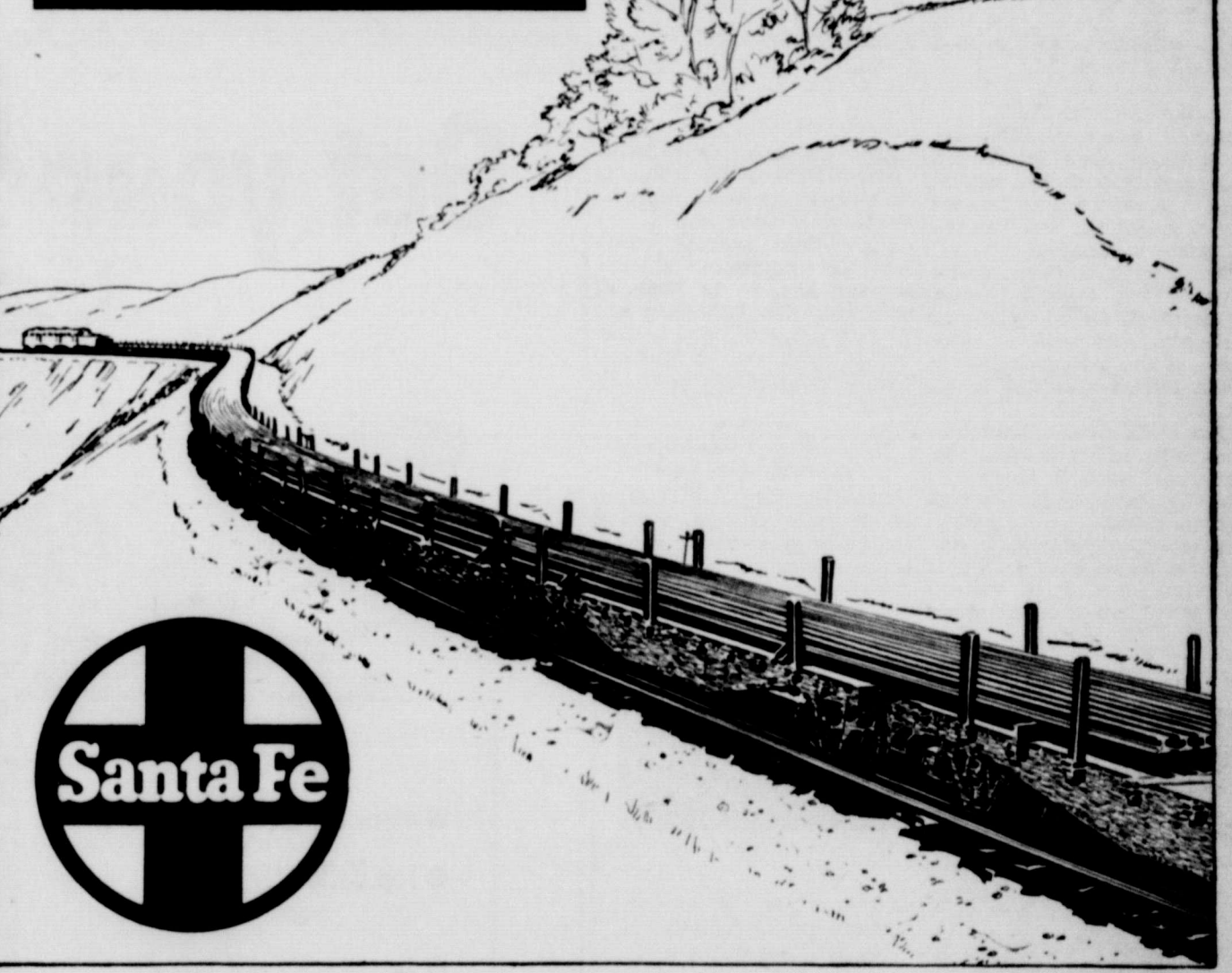
Quarter-mile lengths of welded steel rail curve around a foothill like wire cable.
