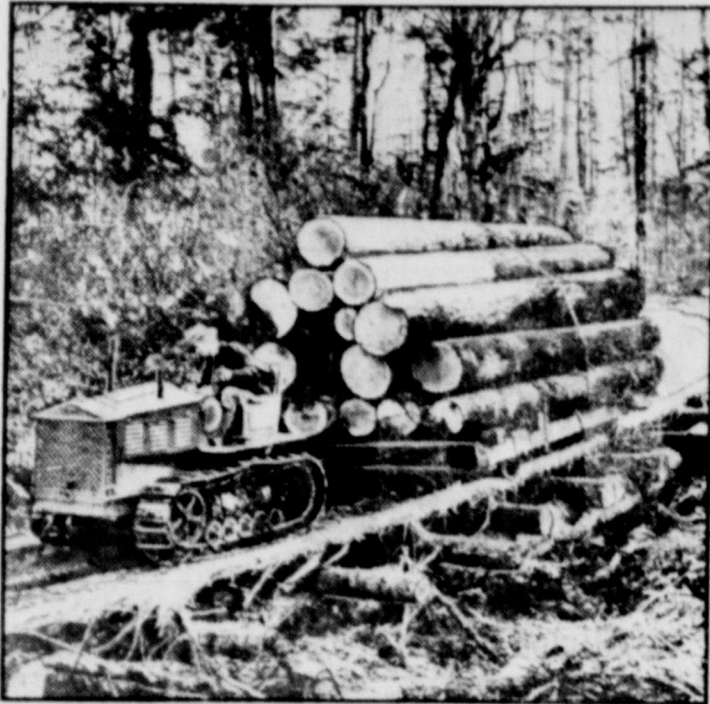
The herculean logging feats performed by the legendary Paul Bunyan seem trivial compared to work done by modern loggers, whose industry has been revolutionized by heavy power machinery. Here a 110-horsepower caterpillar tractor is shown pulling a 10-ton load of logs on a flat car which runs on wooden rails. This scene is from the Naylor logging camp near Ravensdale in western Washington.
