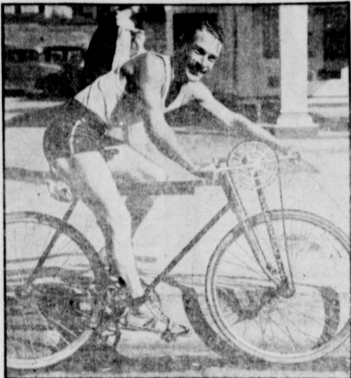
A bicycle that enables riders to exercise both feet and arms, and is said to be capable of a 45-mile-an-hour speed, is pictured above with its inventor, S. J. Hamilton of Los Angeles, in the saddle. With his "exercycle," Hamilton claims he made a round trip to San Diego—a distance of 280 miles—in one day.
