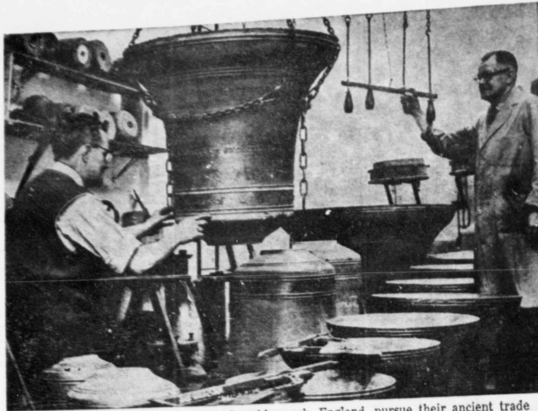
FAMILIAR RING—Technicians in Loughborough, England, pursue their ancient trade of bell-casting. The bells on which they are working are destined for the Episcopal National Cathedral, Washington, D.C. The bells will range in size from a 20-pound bell to a 23,000-pound boomer.
