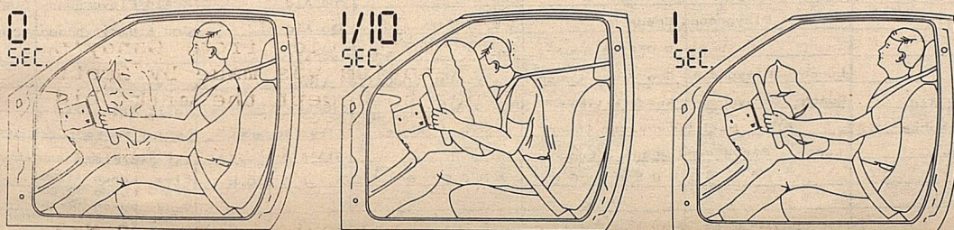
Under normal driving conditions, the air bag is uninflated and packed like a parachute inside the steering wheel hub. When a frontal or near-frontal collision occurs at speeds of approximately 8-12 miles per hour or more, crash sensors trigger the inflator module, causing chemicals sealed inside the module to undergo a reaction and inflate the bag. This cushion splits open the cover of the wheel and protects the driver. The entire inflation sequence takes place in less than 1/10 of a second. After inflation, the air bag automatically begins to deflate in less than one second.
