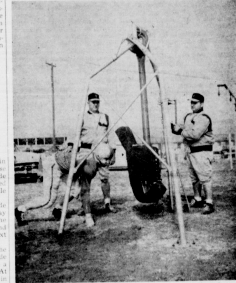
UNKNOWN QUANTITY of pressure will meet the above player when he hits Johnny Truelove's hydraulic blocking machine. The coach (unidentified) will apply the amount of pressure he desires with the control handle. Fifty of the machines being manufactured in Turkey, are on order.
